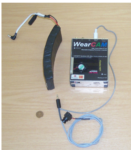
Figure 2 The Complete Capture System (WearCAM Prototype [4] ) one pence piece as size reference. Note Camera (bottom) (See http://www.wear-it.net )
