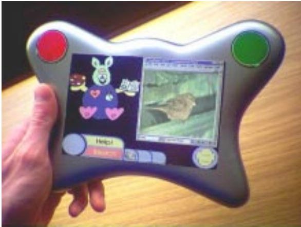
Figure 8. Physical concept model of a children's HandLeR
