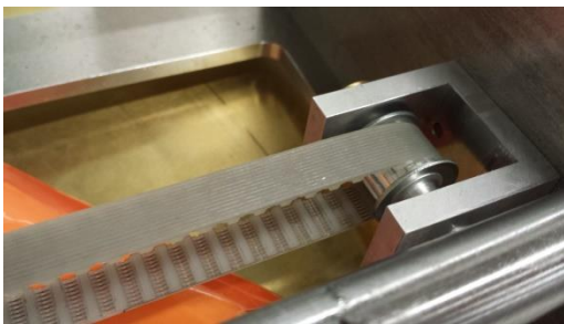
Figure 28 - Toothed belt connected to timing pulley
