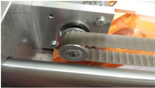
Figure 26 - Timing pulley connected to Y129 stepper motor (same as robot project)
