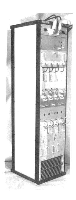
These FM power amplifier bays consist of four 500 watt broad-band modules (AM14/45), each individually fed from an associated switchmode power supply (PS2/281). With an appropriate choice of splitting, combining and harmonic filters, the bay may be configured to give four options:-
